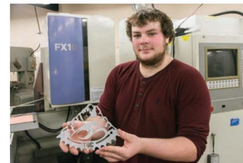
**Penn College manufacturing engineering technology student Joel E. Bergerstock displays one of three emblems he made for The Bicycle Center's Susquehanna River Walk initiative. Bergerstock is standing in front of the electrical discharge machine he used to cut aluminum to form the emblems.**
